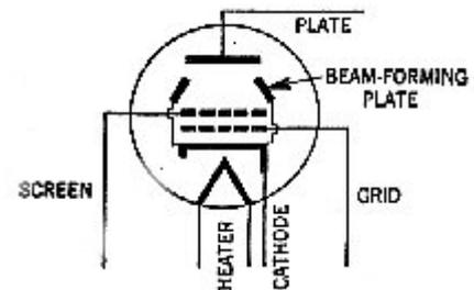
The diagrams on the right show the construction of a beam tetrode output valve and the action of the beam plates in focusing the electron beam onto the anode (plate).
