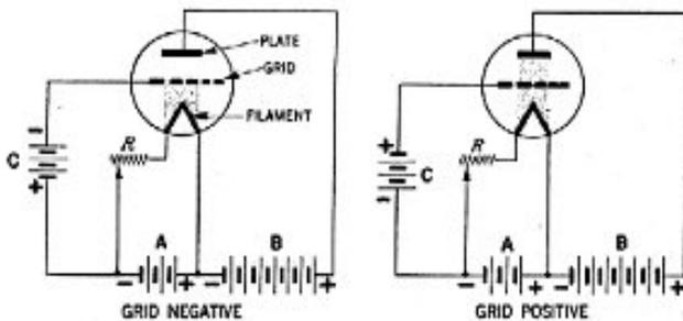
The variable LT resistor 'R' sets the operating voltage, therefore the temperature, of the filament. Although in early days such regulating rheostats were used, they were soon outmoded as advancements were made in valve manufacturing technology.
