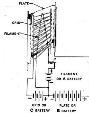
This diagram shows the typical construction of a triode electrode assembly. Note that the filament in this illustration is directly supplying electrons, being heated by the 'A' battery, the grid has a negative potential supplied by the 'C' battery and the anode has an HT potential supplied by the 'B' battery.
